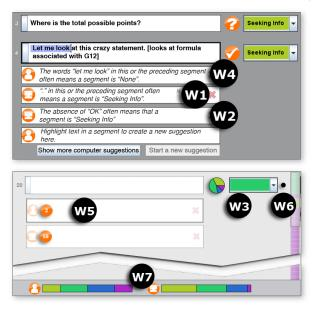
Figure 4: Widgets supporting debugging: Machinegenerated Explanation (W1); Absence Explanation (W2); Prediction Confidence (W3); User-generated Suggestion (W4); Impact Count (W5); Change History Markers (W6); Popularity Bar (W7).
